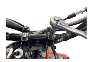
The following parts should be checked periodically for tightness; or if they have been loosened for maintenance, they should be retightened.
